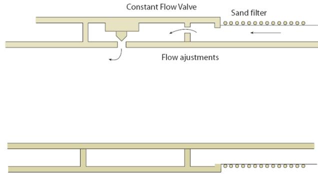
Figure 4: Principle of the BECH autonomous flow control valve.
