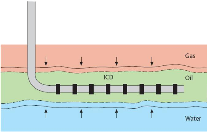
Figure 2: Avoiding coning by applying ICDs.
