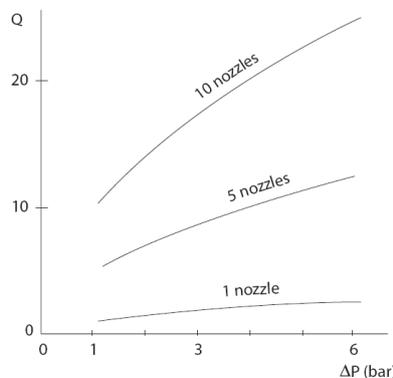
Figure 3: Flow rate – Pressure drop simulations for the FloReg™ ICD. Curves for 1, 5 and 10 nozzles are shown.
