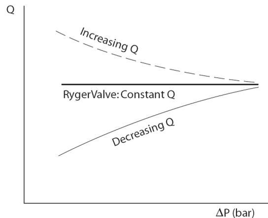
Figure 5: Performance characteristics for the BECH autonomous flow control valve. The horizontal axis is the pressure drop from the reservoir to the production tubing.
