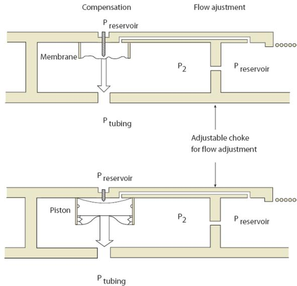
Figure 6: Two designs, upper a membrane, lower a piston.
