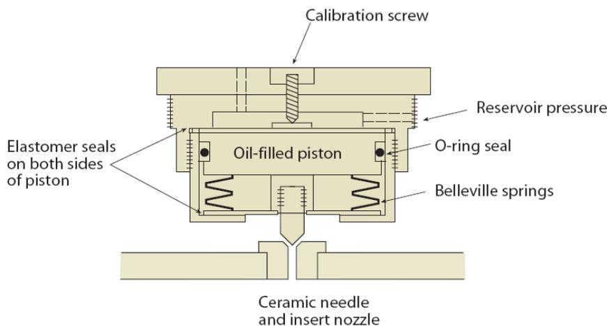
Figure 7: Prototype design of the BECH autonomous flow control valve
