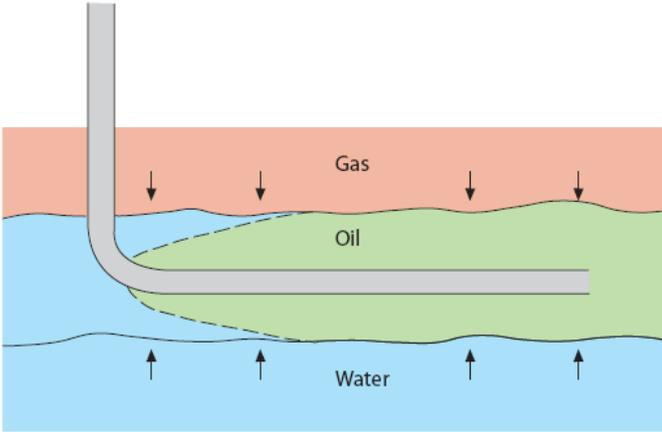
Figure 1: Coning in a long horizontal well.
